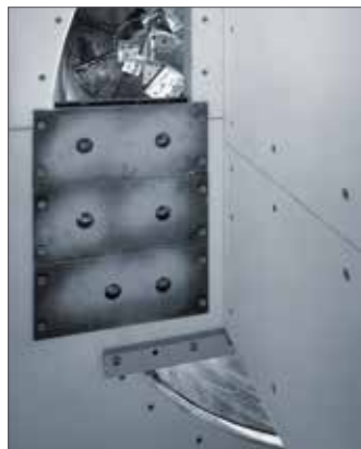
Opening in the end plate with segmented weir and additional bottom discharge
