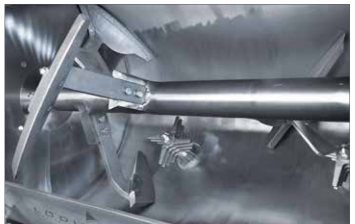
View inside mixing drum
